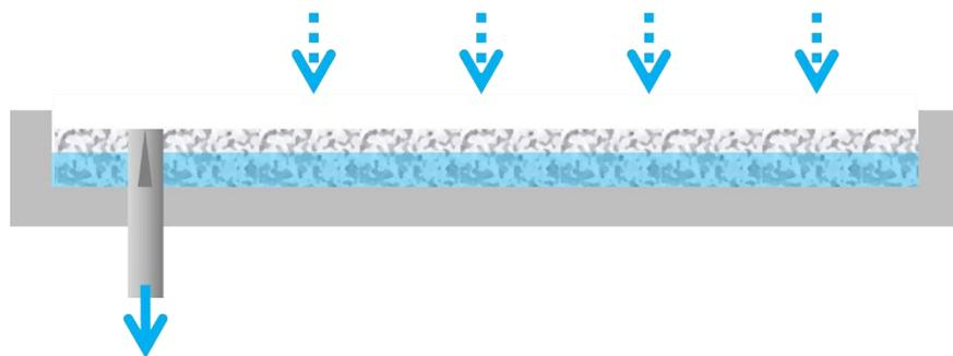
Figure 3 Conceptual diagram of a blue roof where flow control is provided by a shaped weir on the roof leader (shown as triangular notch).
