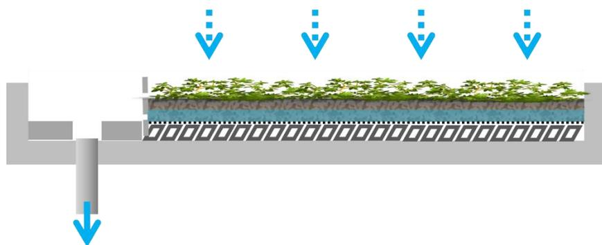
*Figure 4 Conceptual diagram of a green roof where flow control and water storage is primarily provided by the planting medium used to support the vegetation.*
