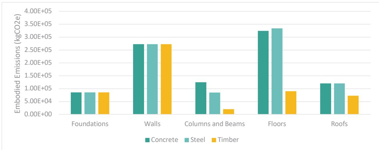
**Figure 7: Embodied Carbon Impacts of Different Structures by Life Cycle Stage**
