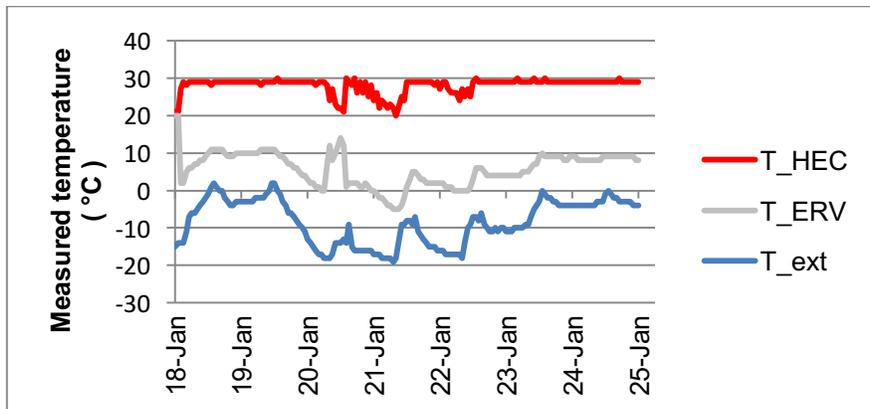
Fig. 2 : Temperature data downstream from the ERV and HEC for January 18 to 24, 2015.
