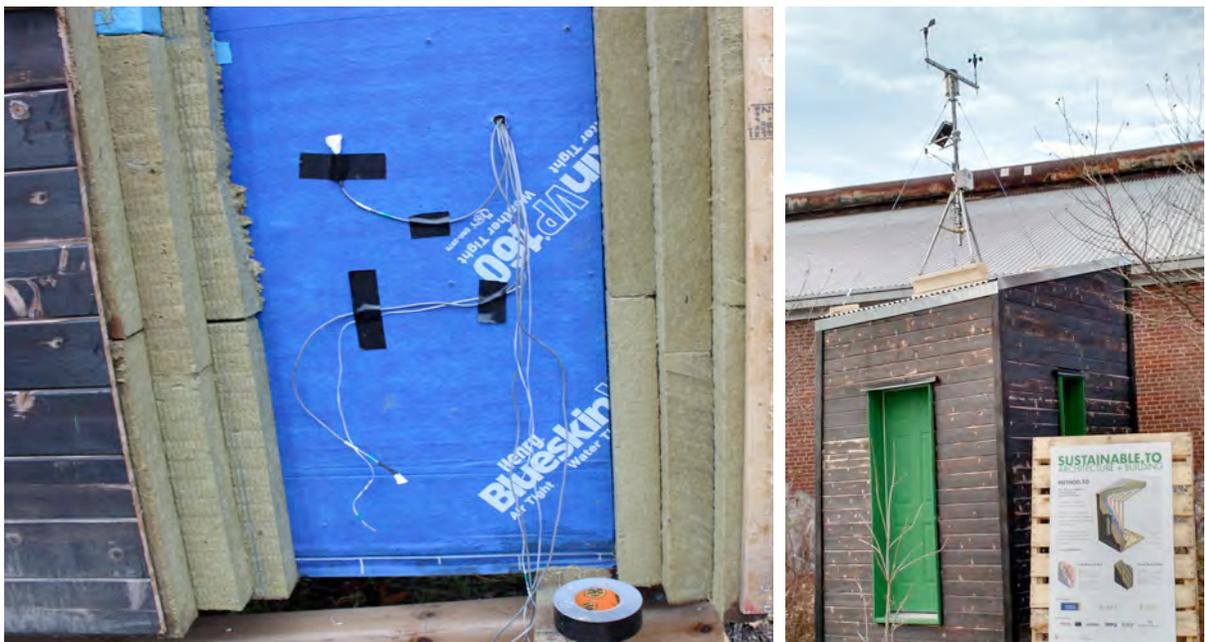
Fig. 2. Sensor Installation; Fig. 3. Test Shed at Evergreen Brickworks with Weather Station.
