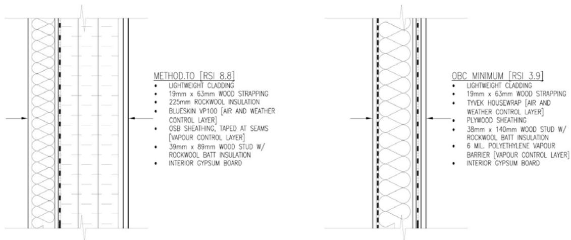
Fig.1. METHOD.TO Construction versus Standard Practice Ontario Code Minimum Construction.
