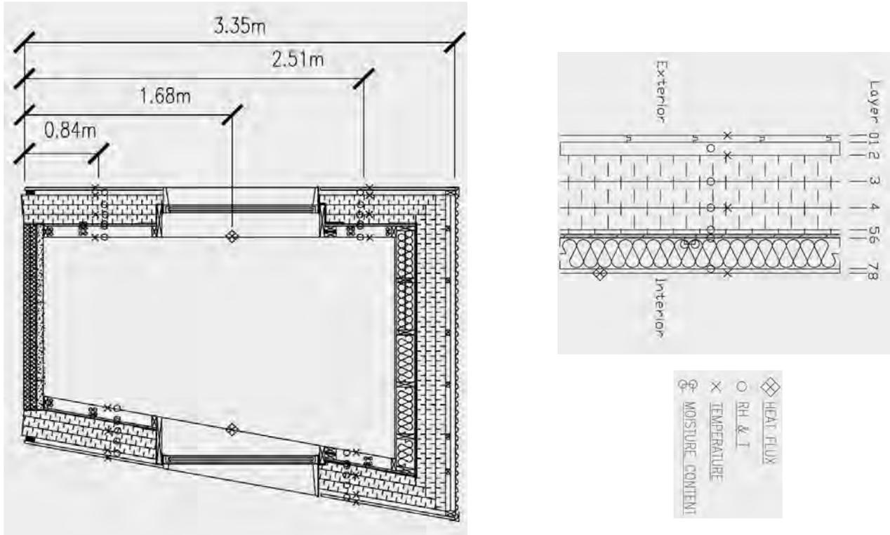
Fig. 4. Sensor Type and Placement Location in the Test Structure.
