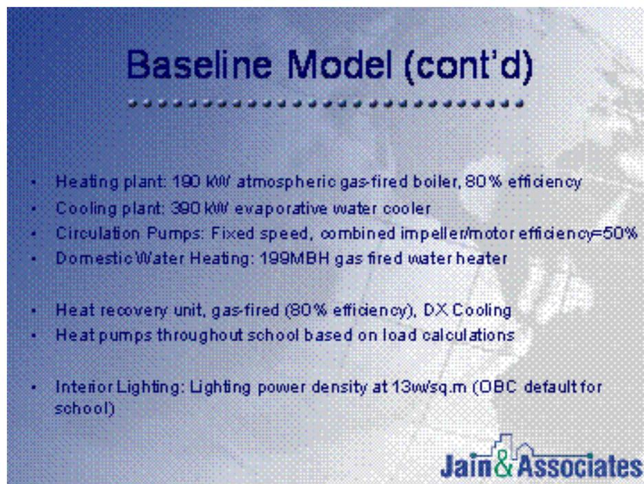
A presentation slide titled "Baseline Model (cont'd)" with a dotted line separator. The slide lists details of the heating and cooling plants, circulation pumps, domestic water heating, heat recovery, and interior lighting. The Jain & Associates logo is in the bottom right corner.
