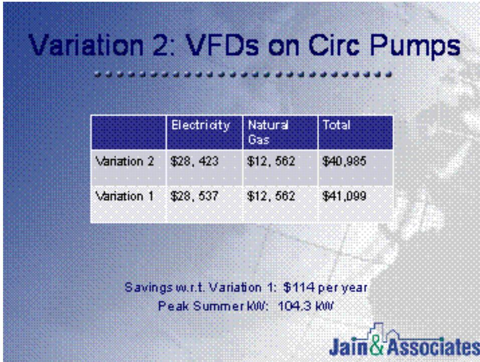
Figure 6. Alternative 3. Variable Frequency Drives on Circulation Pumps
