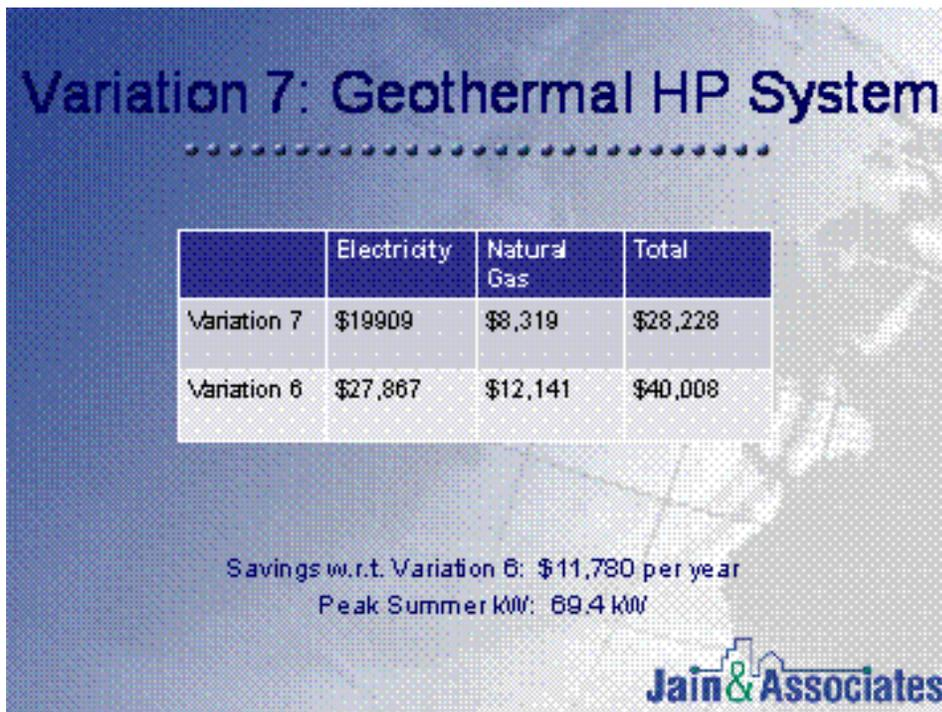
The team noted the criticality of the installation (or not) of a central air conditioning system. This choice affects related choices with respect to the heating system. In particular, the use of geothermal is only “worth it” if there is central air conditioning. Similarly, thermal heating (e.g. in floor radiant heating) will likely be precluded if central air conditioning is selected.
