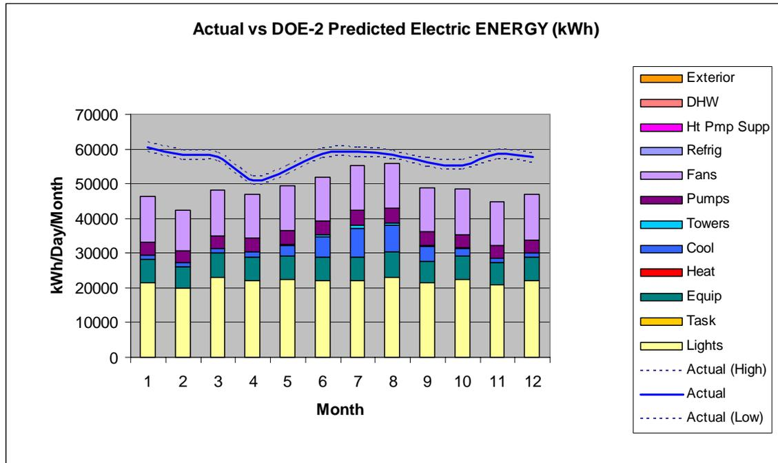
*This graph shows the model build up of the energy uses in the building (column graph) compared with the actual electrical consumption (blue line). There is a “winter extra” electrical load currently not included in the model – this is partly attributed to the rink refrigeration plant, and partially due to electric heating in the building.*
