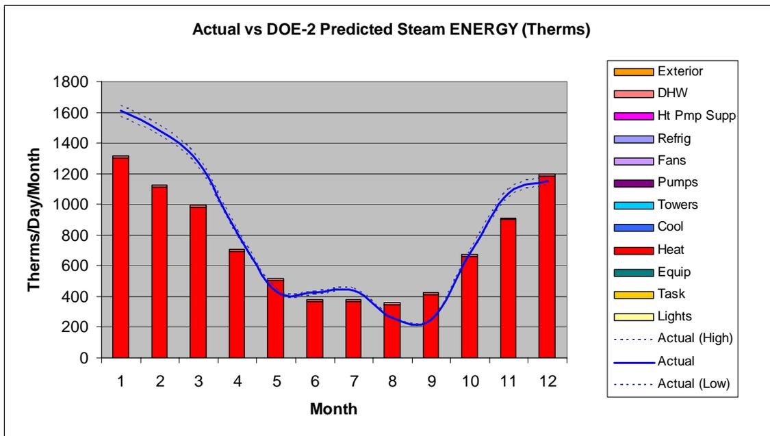
*Steam use for the building compared with the model prediction. There is significant summer steam use in this facility. Very little of this goes to DHW heating – most of it goes to heating in the dual-duct units and to reheating already cooled air.*
